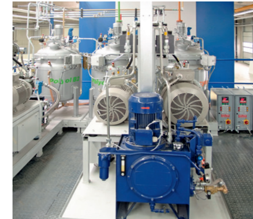
Fully automated high-pressure dosing machine for PUR-foam
