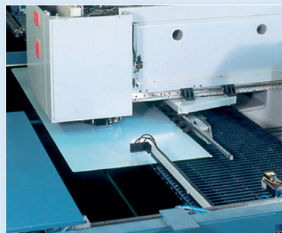
CNC-controlled sheet metal processing line for cutting to size, punching and bending sheet metal
